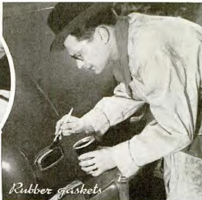
Dust cannot enter the carburetor air cleaner and the crankcase-ventilator inlet and outlet openings if paper bags are tied over them. Rubber gaskets should be protected by coating them with special paint
